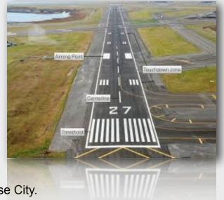
"The runway heading sets up with the magnetic and with the compasses and all the instruments that are in the aircraft," Klein said. "So we want to make sure that those line up appropriately." The Gaylord Regional Airport is currently about six degrees off, and that number could get up to 10 degrees.
